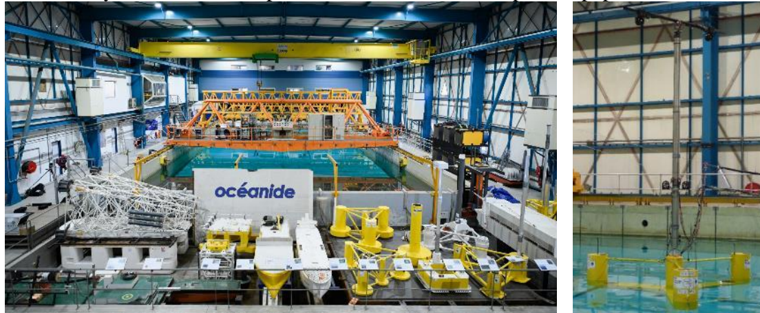
Figure 8. South France Ocean Basin (left) and VoltturnUS floater with 15MW turbine (right)
