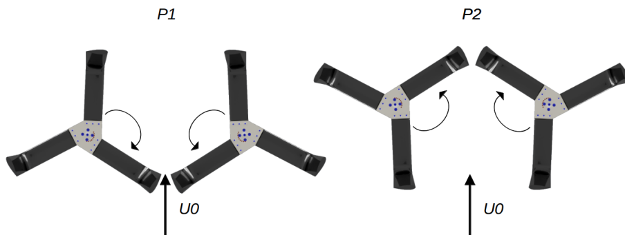
Figure 2: Schematic view of the two rotational directions of the counter-rotating rotors.
