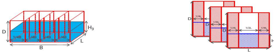
Figure 2: ART geometry. Each solidity ratio is equal to 50% (ratio of the area of the baffle to the total area ART section) (3D view and section details).
