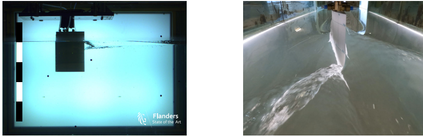
FIGURE 2 – Test in freshwater at \beta = -10^\circ , Fr_T = 0.96
