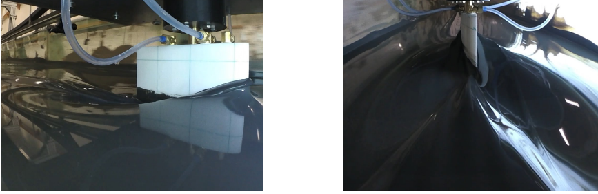
FIGURE 4 – Experiment in condition A at Fr_T = 0.96 , \beta = 5^\circ (left), and \beta = -5^\circ (right)
