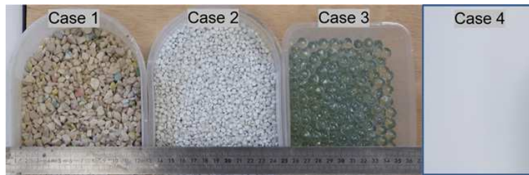
FIGURE 6 – Granular media : small rocks (case 1), PVC pellets (case 2), glass balls (case 3), foam (case 4).
