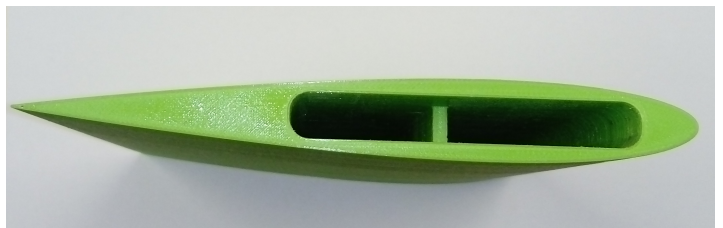
(b). 3D printing NACA 0012 with fairing system
