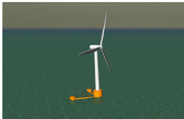
Figure 2 - Floating wind turbine modelling in OrcaFlex
