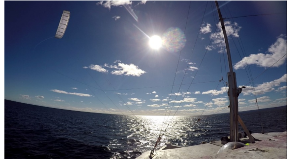
Figure 5 – beyond the sea® kite of 50 m 2
