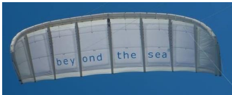
Fig. 1: Kite used during measurement. C-shape with inflatable leading edge and battens, 50m 2 , 23 kg (deflated, with bridles and tethers).
