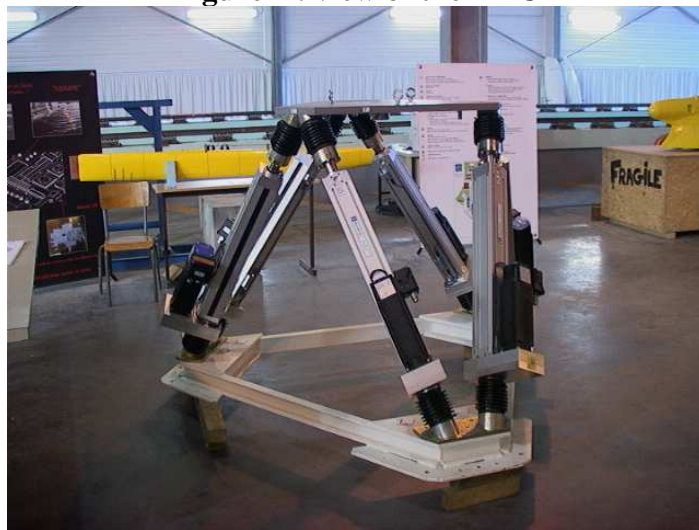
Figure 2 : hexapod – a 3D motion generator
